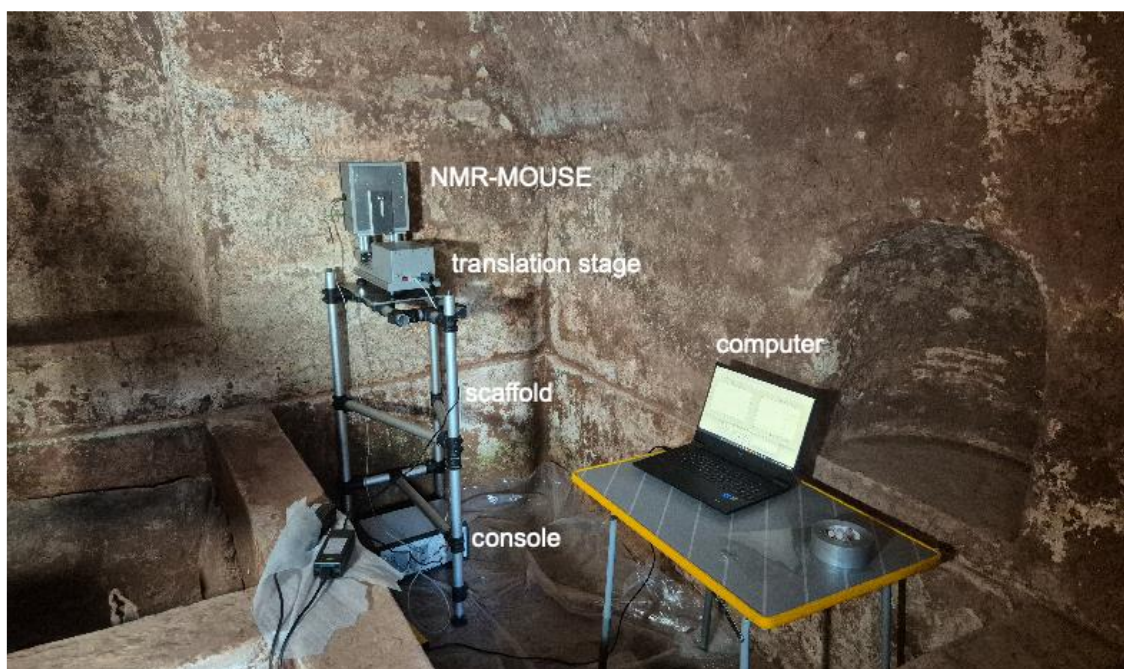
Figure 1: NMR setup for measuring depth profiles. The NMR-MOUSE is mounted on a precision translation stage, which rests on an adjustable scaffold. The sensor and the translation stage are connected to the console, which is operated by the computer.
