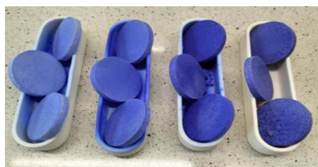
Fig. 2: Synthesized Co-SP with increasing cobalt content. Visual appearance reflects varying degrees of Co 2+ incorporation into the SP matrix structure.
